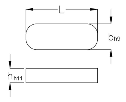
$\begin{array}{ll} b & = 8 \\ h & = 7 \\ L & = 80.0 \\ Tolerance \ b = 0.036 \\ Tolerance \ h = 0.090 \\ Tolerance \ L = -0,3 \end{array}$
